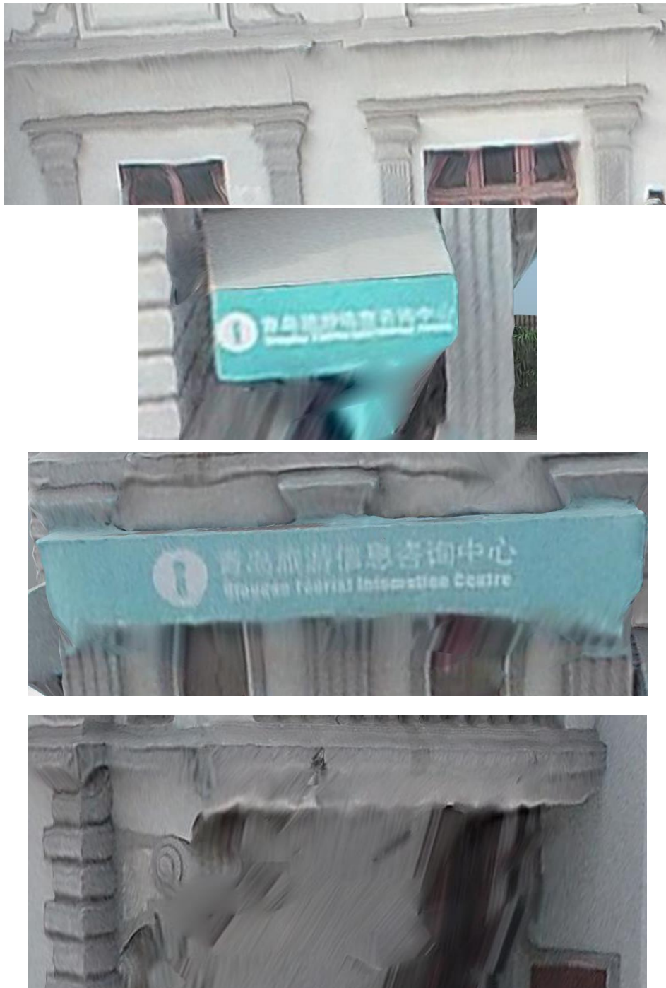
Figure 8 UAV aerial image reconstruction model problem
