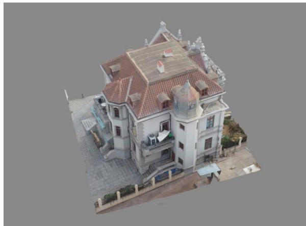
Figure 7 3D Real Scene Model rendering of UAV aerial images
